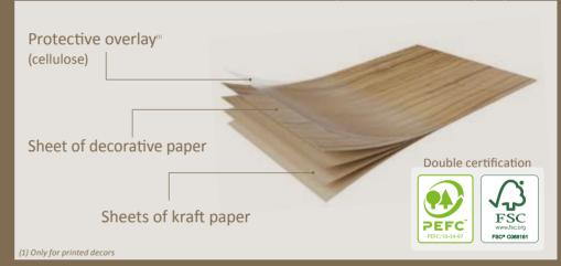
As a wood-based product, the High Pressure Laminate uses natural resources for almost 65% of its composition. The remaining 35% are thermosetting resins which comply with the requirements of REACH<sup>(1)</sup> regulations in respect of chemical substances.
